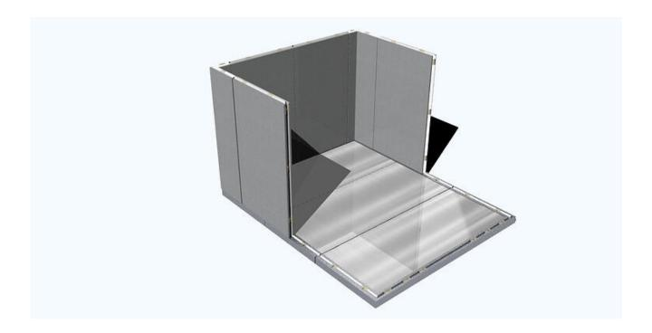
**Step 4**: Assemble your first ceiling panel. Start by aligning the end ceiling panel with the corners of the wall panels. The tongue-n-groove will hold the ceiling panel in place.
