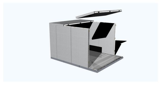
**Step 7**: Continue assembling wall panels and ceiling panels as per your assembly drawing. The last wall panel assembled should be a front corner panel.
