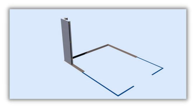
**Step 4**: Place a wall panel on each side of the corner panel and firmly fasten the wall panels to the corner panel using a hex wrench or drill. Make sure the top of the panels are flush and level before firmly fastening the cam locks.
