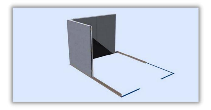
**Step 5**: Continue assembling vinyl screeds and wall panels as per your assembly drawing. Work your way around the box as per the rendering below. This provides stability as you build your box.
