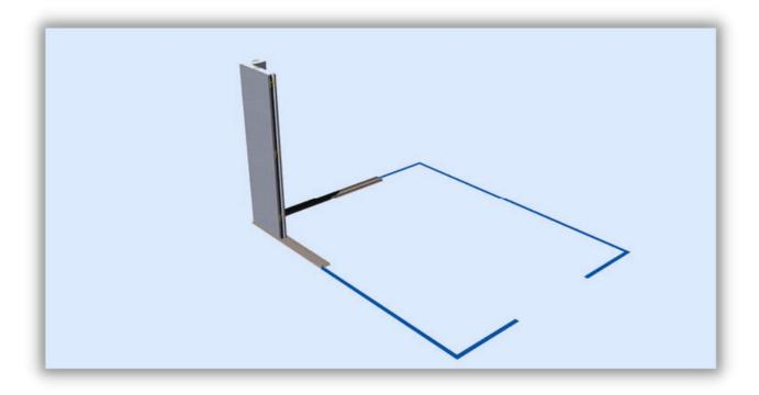
**Step 3**: Continue adding vinyl screeds in both directions as per your assembly drawing, repeating step 1 as you do. Make sure your floor remains level as you assemble each additional screed.
