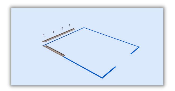
**Step 2**: Start panel assembly by placing a corner wall panel in the corner screed.
