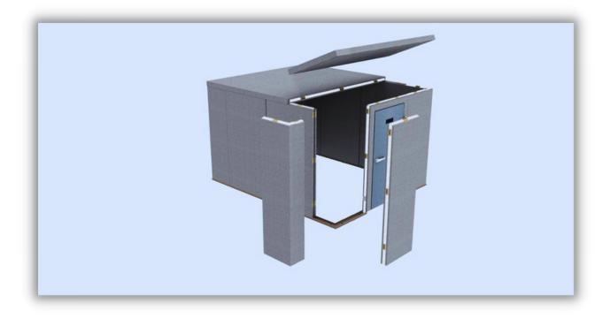
**Step 11**: Firmly fasten the ceiling panels to the top of the wall panels once all your screeds and panels are assembled and level at the top.
