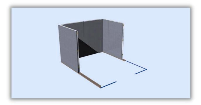
**Step 6**: Start ceiling panel assembly with the end ceiling panel as per your assembly drawing. Align the ceiling panel with the corners of the wall panels. The tongue and groove method will hold the ceiling panel in place.
